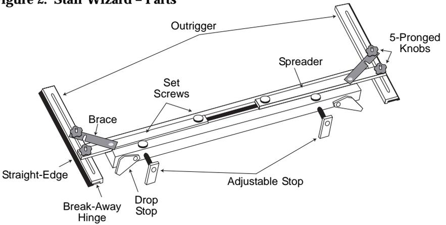
**Figure 3. Setting The Adjustable Stops**
